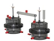
Corrolytics' test kit uses UA technology to better diagnose the cause of corrosion
